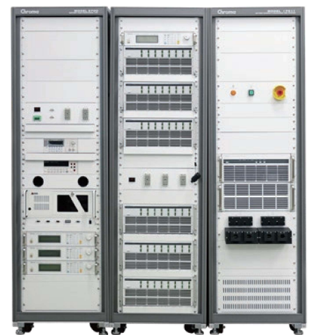
Distributed BMS test system (96S)
