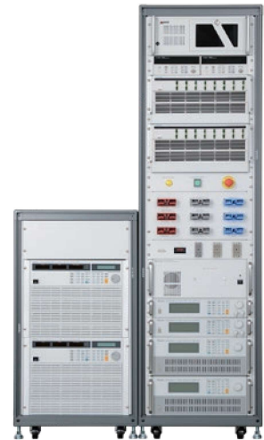
Integrated BMS test system (32S)
