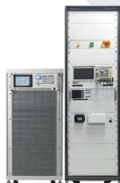
EV Wireless Charger ATS
